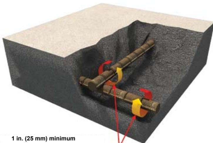
**1 in. (25 mm) minimum clearance between reinforcement and existing shotcrete**
