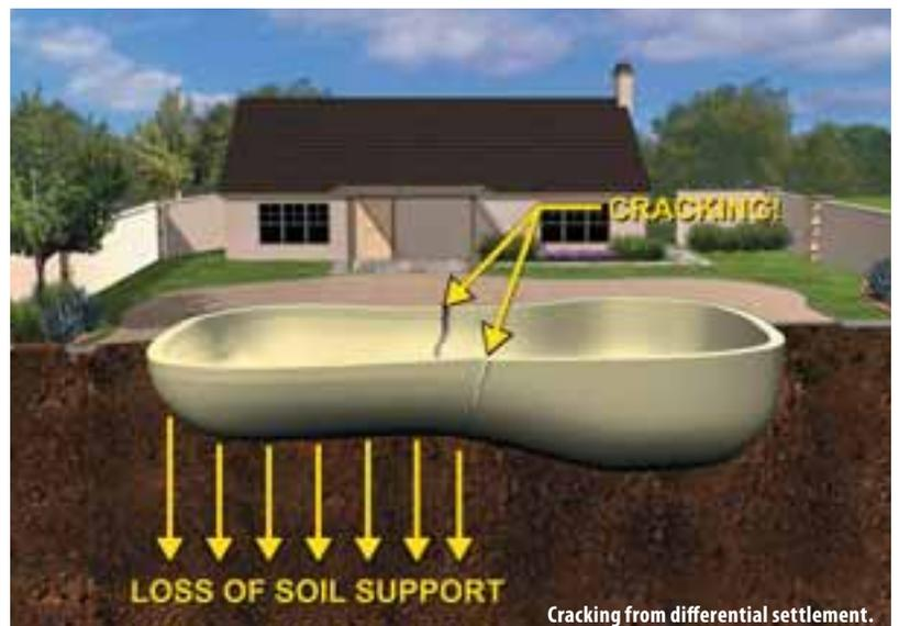
But a pool varies from a retaining wall in that it often holds 200,000 pounds or more of water in addition to the pressure from surrounding soil. If the soil under a portion of the pool doesn't support the pool, that area of the pool will settle. When a portion of the pool settles while the remainder of the pool is properly supported and does not settle, it is called differential settlement – which frequently results in cracking of the pool.
